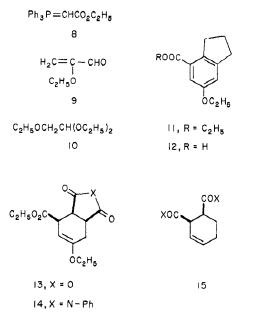
The conditions used lead to ester hydrolysis, and the product was isolated as the parent acid 12. Reaction of diene 7 with the active dienophiles maleic anhydride and N-phenylmaleimide at 110° yielded the nicely crys-talline cyclohexenes 13 and 14. The related condensation of vinylacrylic acid with acrylic acid and that of
